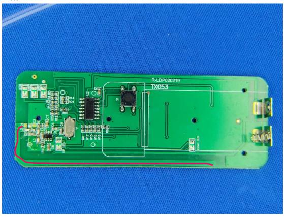
Antenna Gain: PCB antenna with maximum gain 0 dBi
