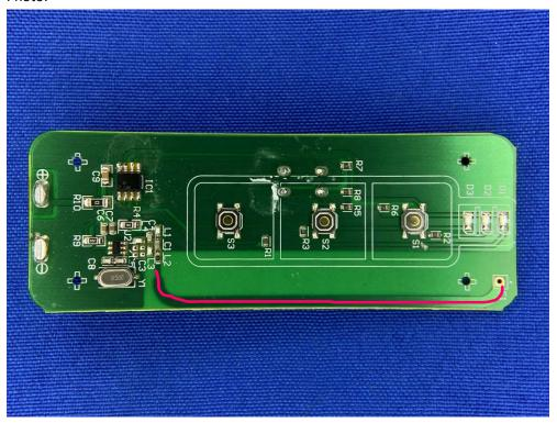
antenna Gain: PCB antenna with maximum gain 0 dBi
