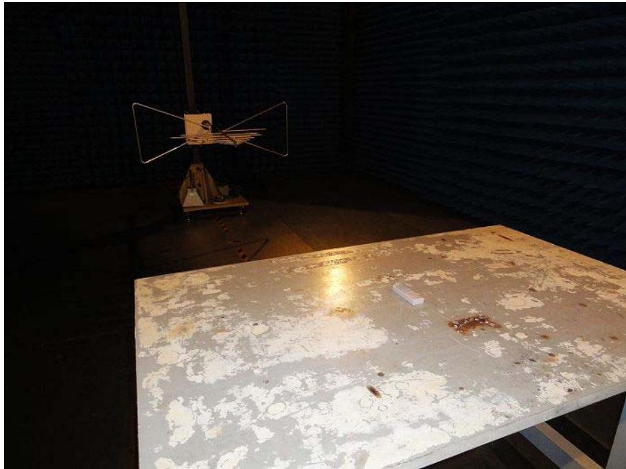
Radiated emission test view
