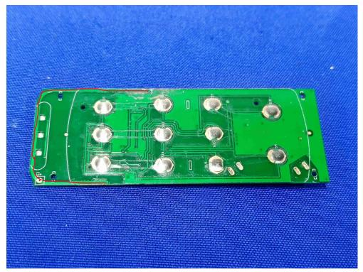
Antenna Gain: PCB antenna with maximum antenna gain 0 dBi
