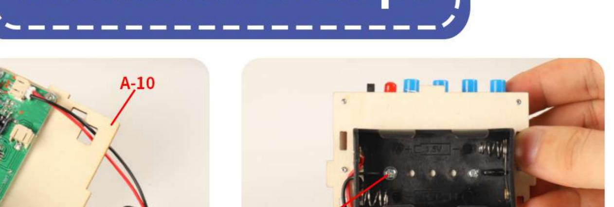
20. flip it over, align the battery box with 19. Pass the battery box wires through the the screw holes, and secure it with 4MM screws as shown in the diagram.
