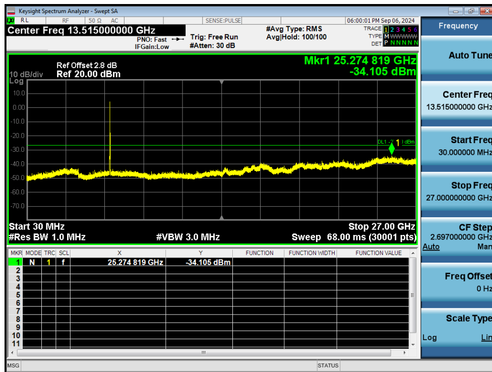
Tx. Spurious NVNT ac20 5785MHz Ant1 Emission
