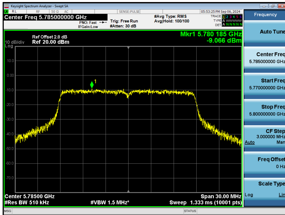
PSD NVNT n20 5785MHz Ant1
