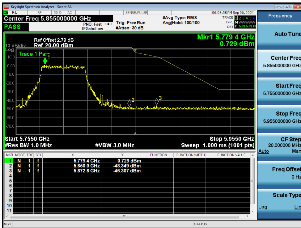
Band Edge NVNT ac40 5795MHz High Ant1
