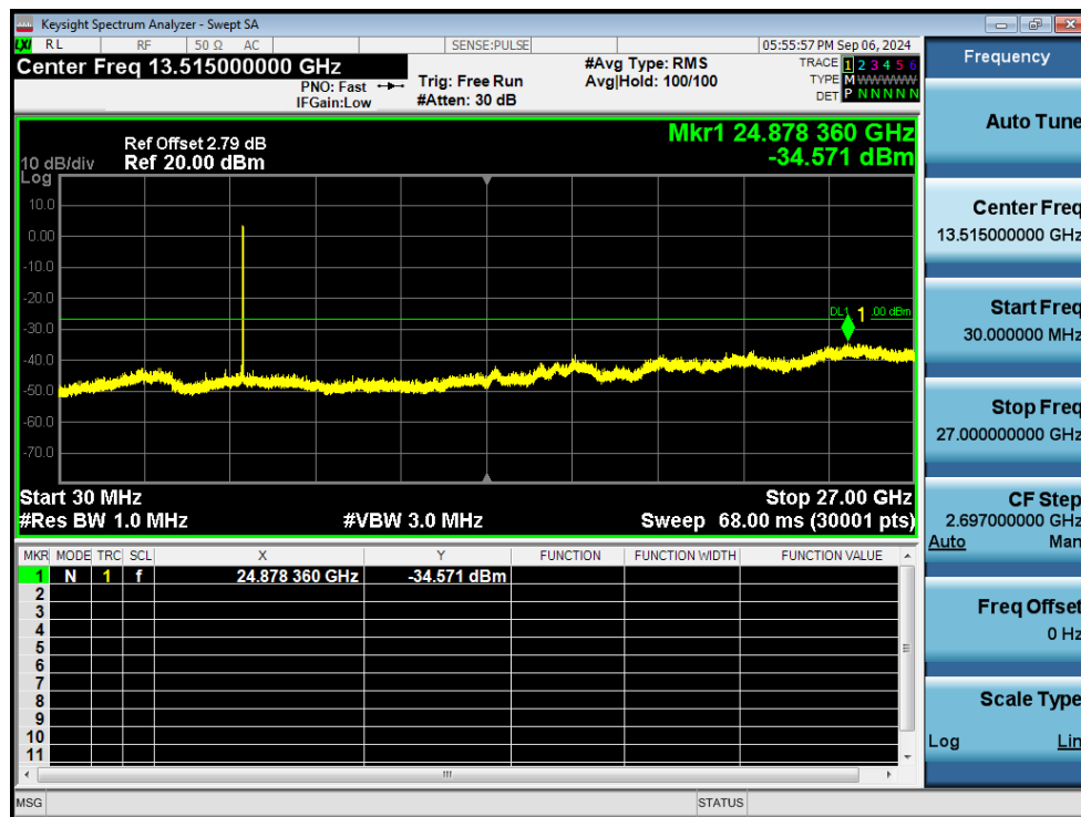
Tx. Spurious NVNT n20 5825MHz Ant1 Emission
