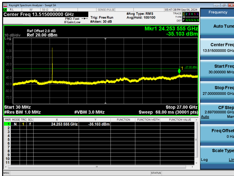
Tx. Spurious NVNT a 5785MHz Ant1 Emission
