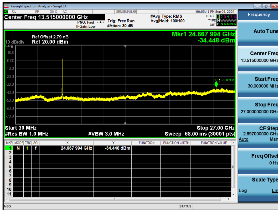
Tx. Spurious NVNT n40 5795MHz Ant1 Emission
