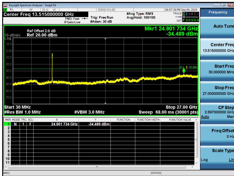
Tx. Spurious NVNT ac80 5775MHz Ant1 Emission
