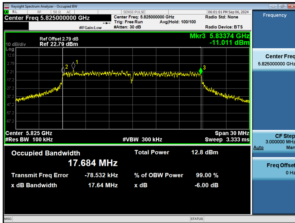
-6dB Bandwidth NVNT ac20 5825MHz Ant1
