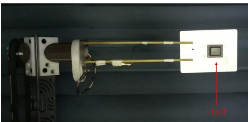
FIGURE4.1.3 ANTENNA TEST PICTURE WITH OTA CHAMBER
