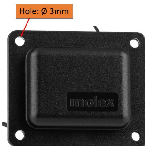
FIGURE 5.2 ANTENNA HOLE MOLEX DOES NOT RECOMMEND SCREW MODELS, BUT IT IS RECOMMENDED TO ADD A GASKET WHEN USING SCREWS.
