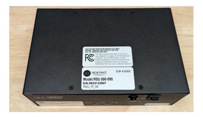
**NOTE:** The label affixed to the device is printed on a highly adhesive sticker. This sticker is designed to bond firmly to the device, ensuring that it cannot be removed easily. Removal of the sticker requires the assistance of a blade or other mechanical means, guaranteeing that the label remains securely attached under normal usage conditions.
