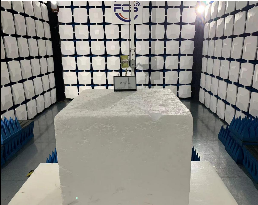
Above 1GHz for radiated emission test setup
