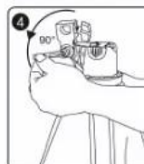
STEP 4 Loosen the knob on the softbox, turn 90° and lock it
