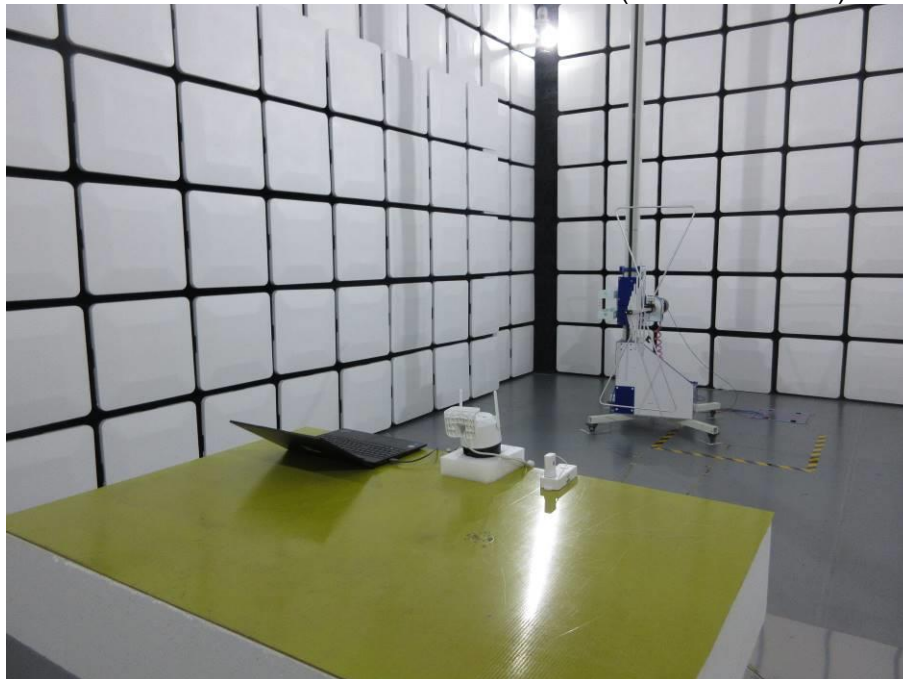
RADIATED RF MEASUREMENT SETUP (30MHz ~ 1 GHz)
