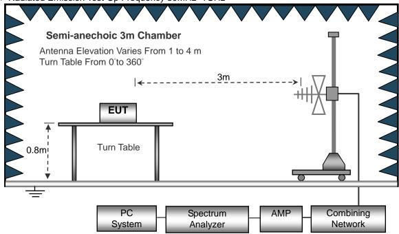
(C) Radiated Emission Test-Up Frequency Above 1GHz
