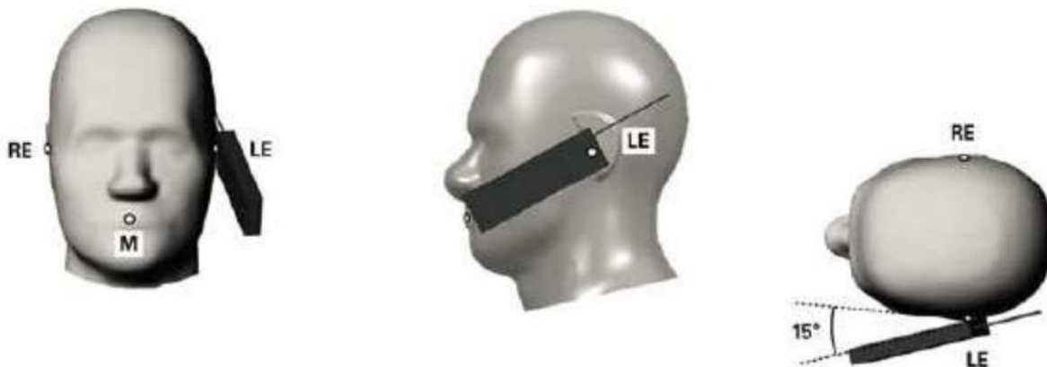
Fig.8-4 Illustration for Tilted Position
