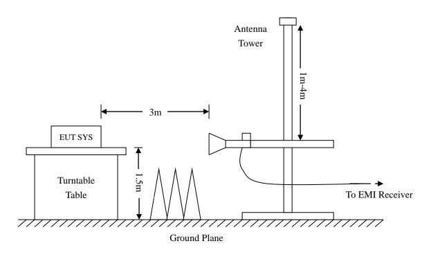
Frequency :9kHz-30MHz Frequency :30MHz-1GHz Frequency :Above 1GHz
