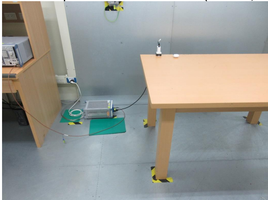
Photograph 16: Test Setup for Mains Conducted Emissions (Front View, Charge Mode)
