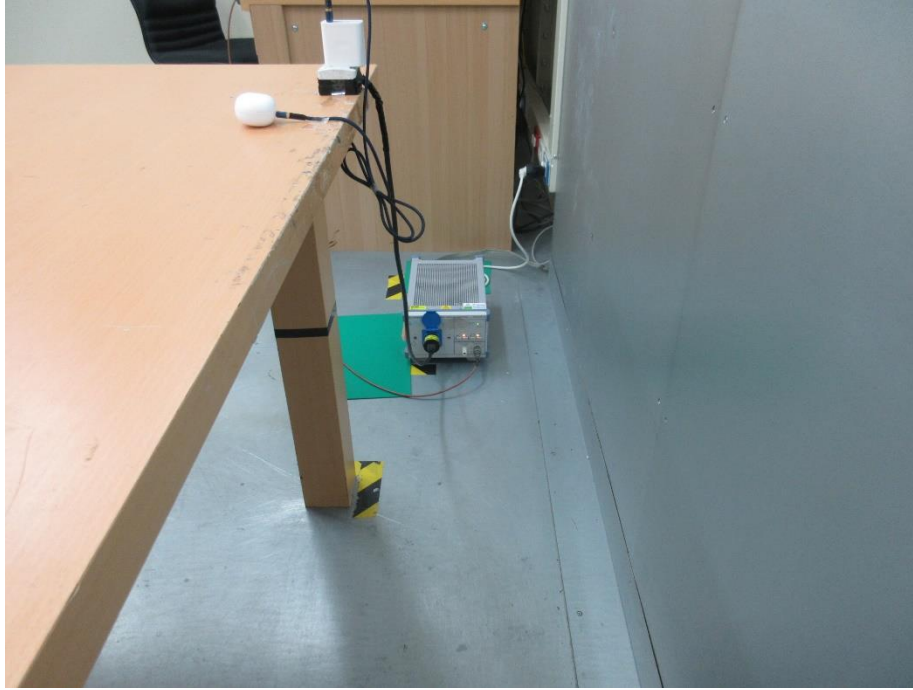
Photograph 17: Test Setup for Mains Conducted Emissions (Back View, Charge Mode)
