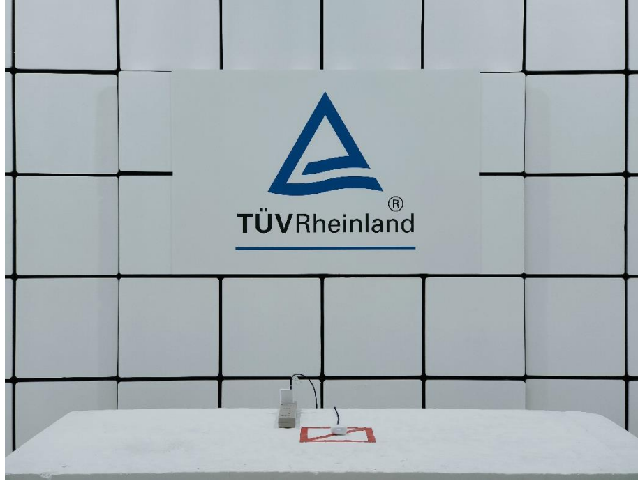
Photograph 14: Test Setup for Spurious Emissions (Back View 1, Charge Mode)
