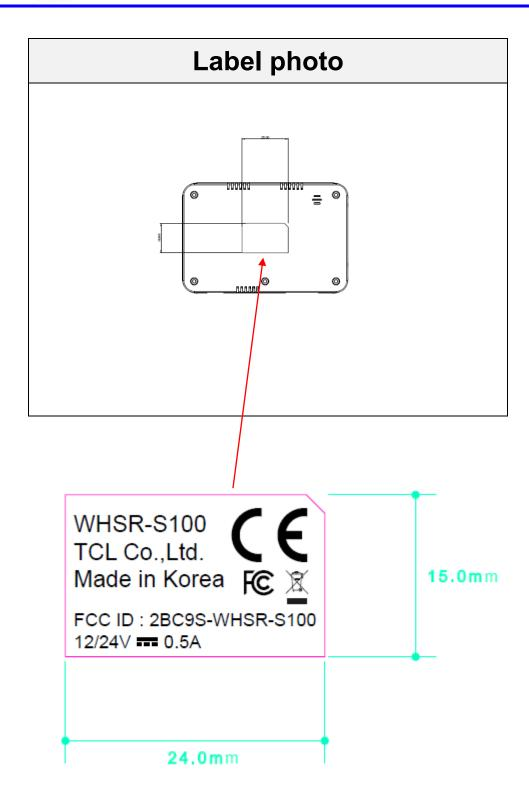
The device is so small that it is not practicable to place the statement specified under 15.19 statement request, the information required by this paragraph shall be placed in a prominent location in the User's Manual.
