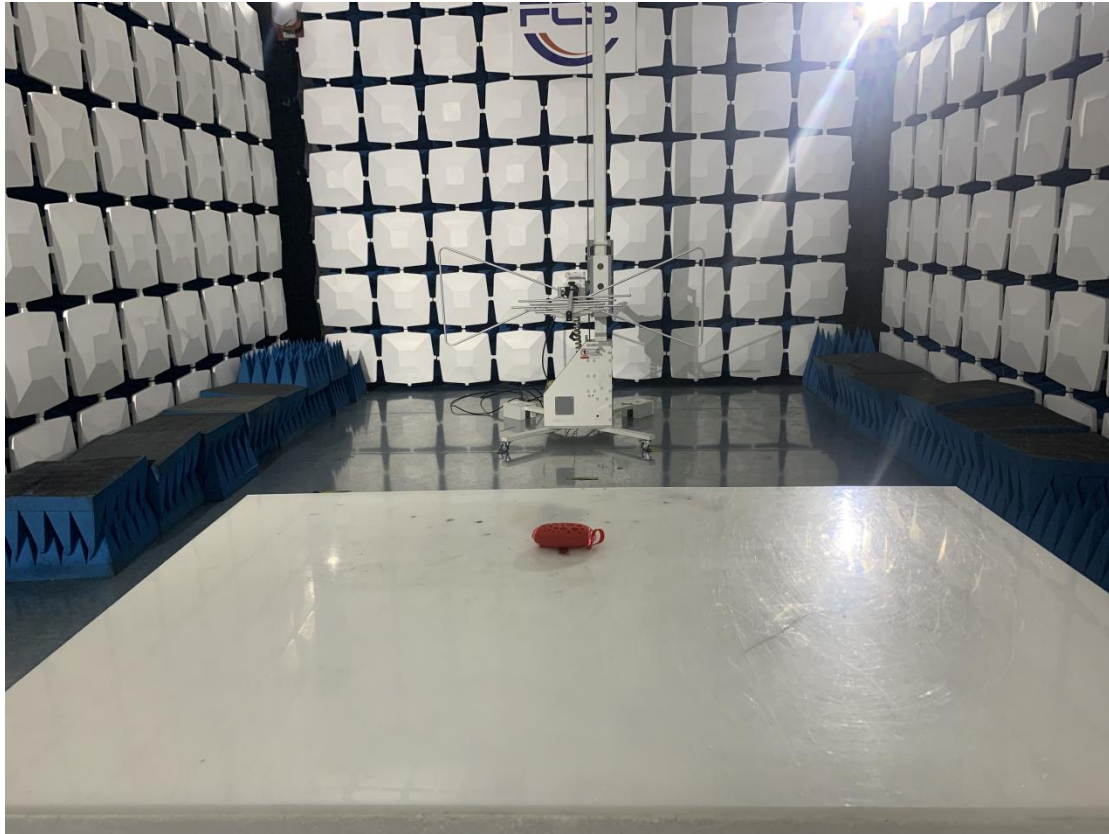
Blow 1GHz for radiated emission test setup
