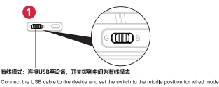
有线模式: 连接USB至设备, 开关拨到中间为有线模式 Connect the USB cable to the device and set the switch to the middle position for wired mode.
