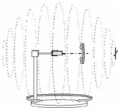
图（2）手机在暗室内三维定位装置 Figure (2) Three-dimensional positioning device for mobile phones in a dark room
