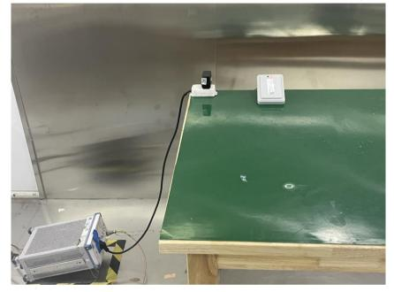
RF Radiated Test (30MHz-1GHz)
