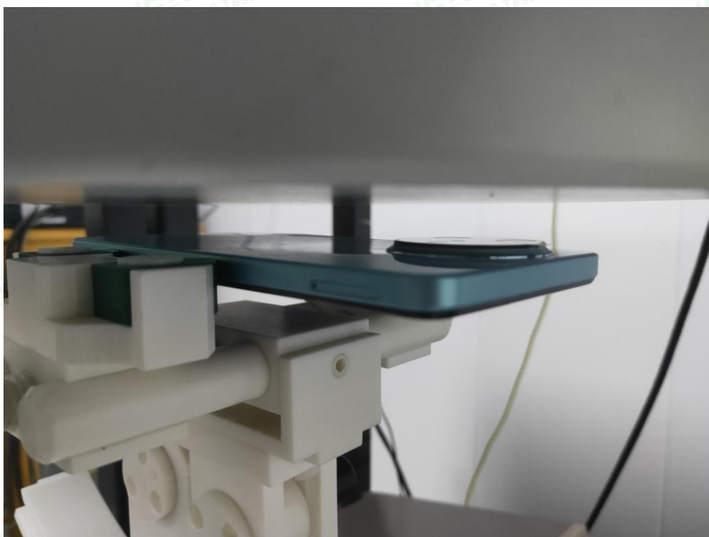
10mm body-worn Back Side Setup Photo (hotspot)
