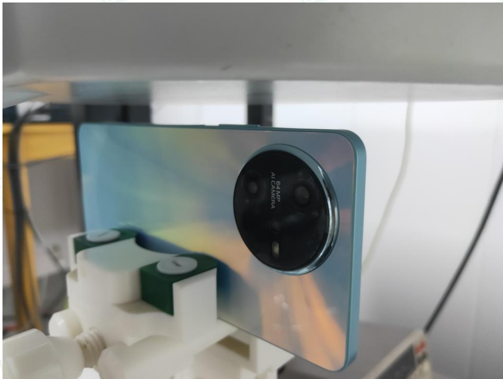
10mm body-worn Right Side Setup Photo (hotspot)
