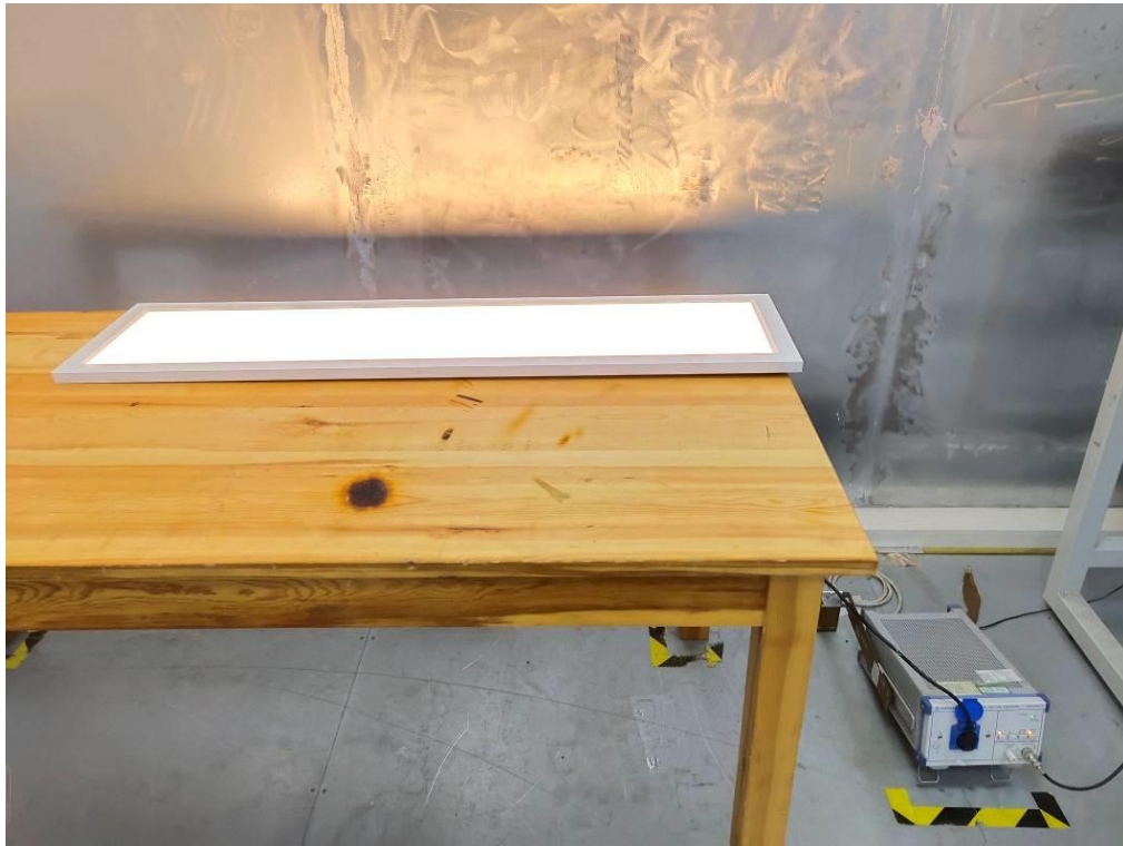
Photo of Power Line Conducted Measurement
