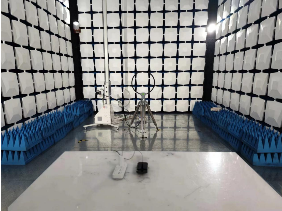
Blow 1GHz for radiated emission test setup
