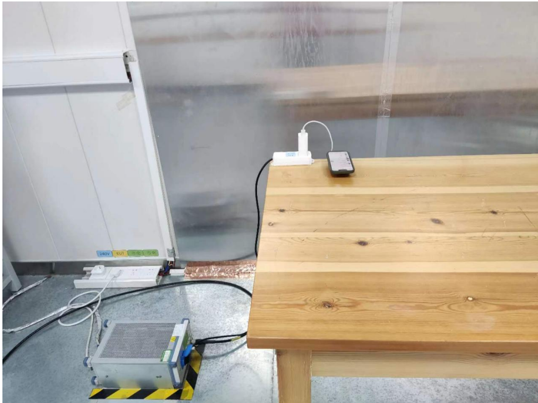
Conducted emission test setup
