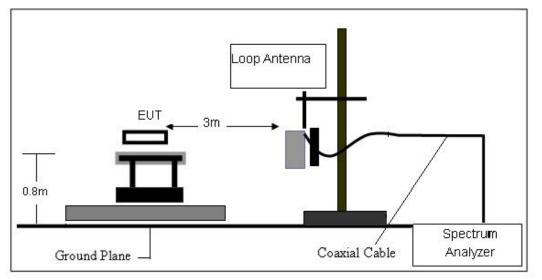
(B) Radiated Emission Test-Up Frequency 30MHz~1GHz
