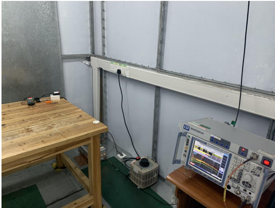
Test Setup For Conducted Emission
