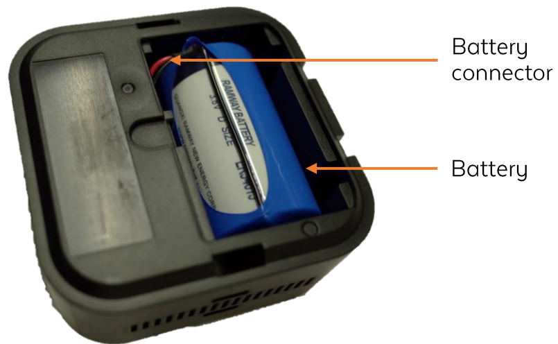
Figure 2-3 UPIDO basic bottom inside view
