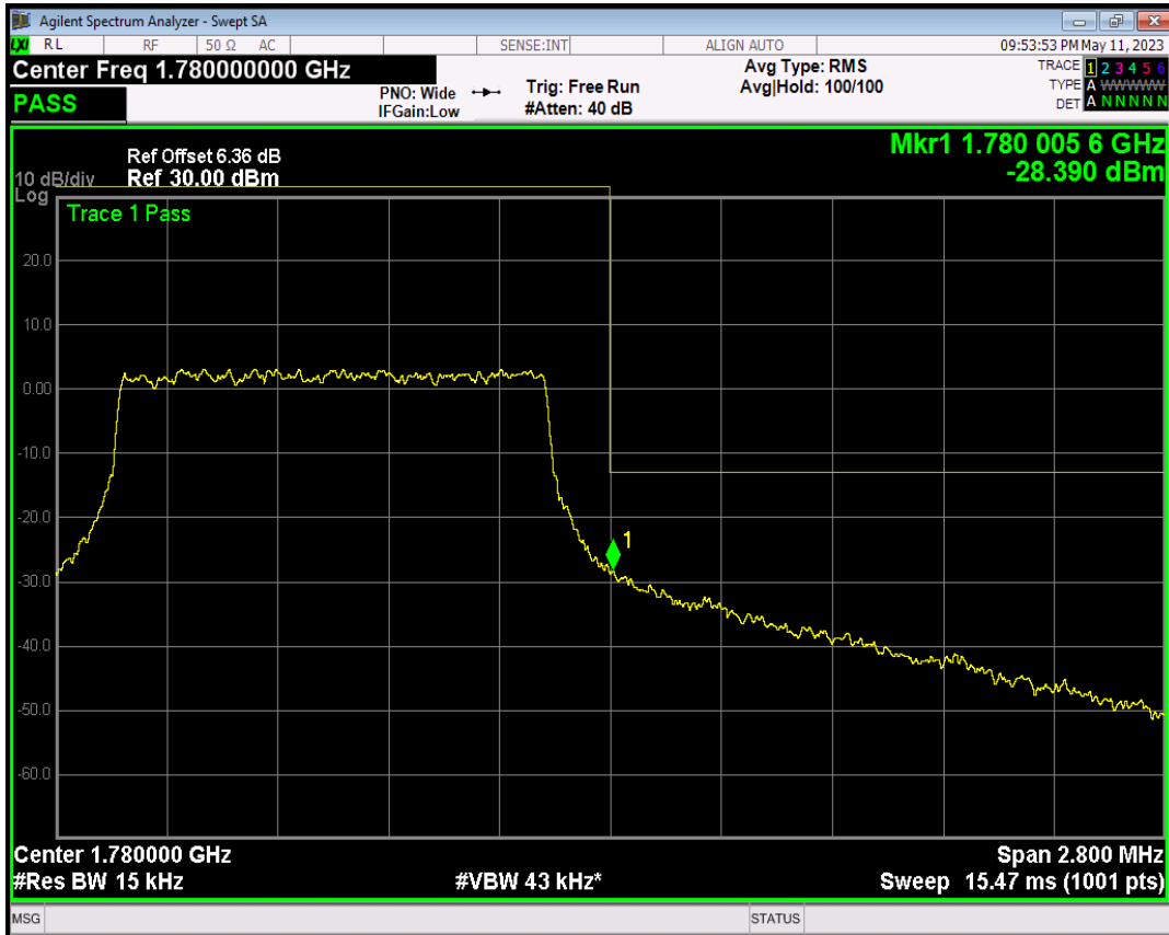
Band66 QPSK BW=3MHz Channel=131987 RB Size=15 Position=#0
