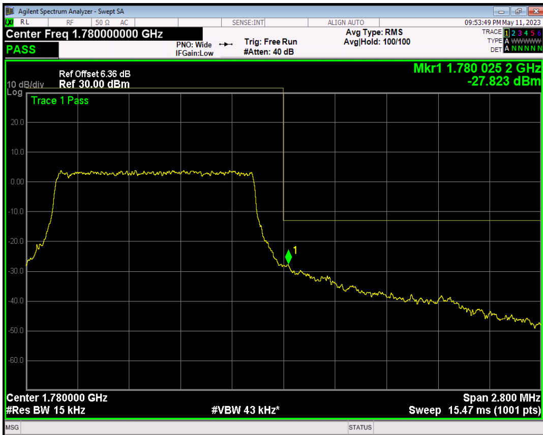
Band66 16QAM BW=1.4MHz Channel=132665 RB Size=6 Position=#0
