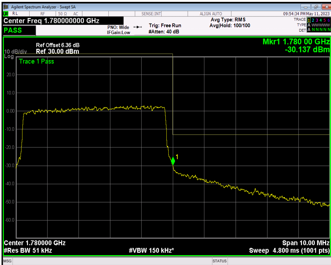
Band66 16QAM BW=5MHz Channel=132647 RB Size=25 Position=#0
