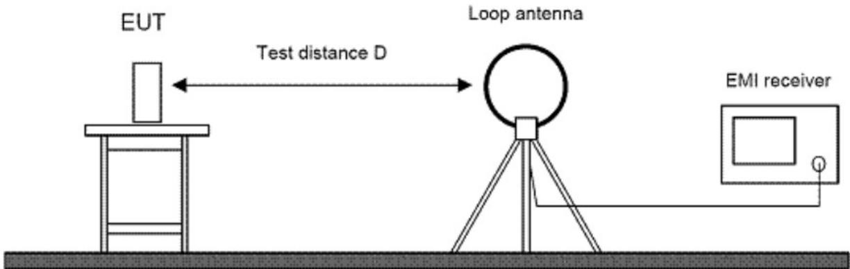
**Figure 4. Radiated Emissions Test Setup (9kHz - 30MHz)**
