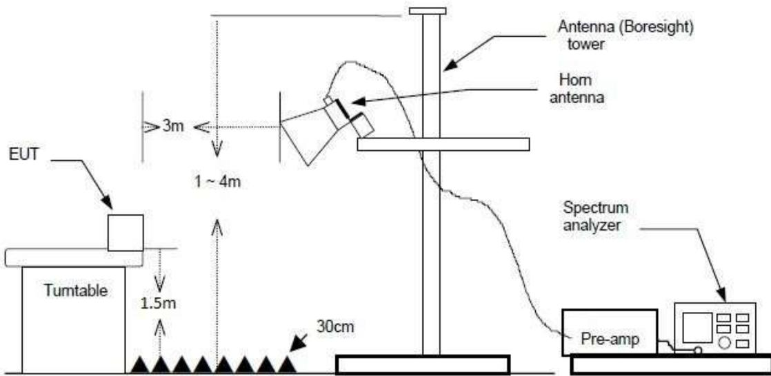
**Figure 5. Radiated Emission Above 1GHz Test Setup**
