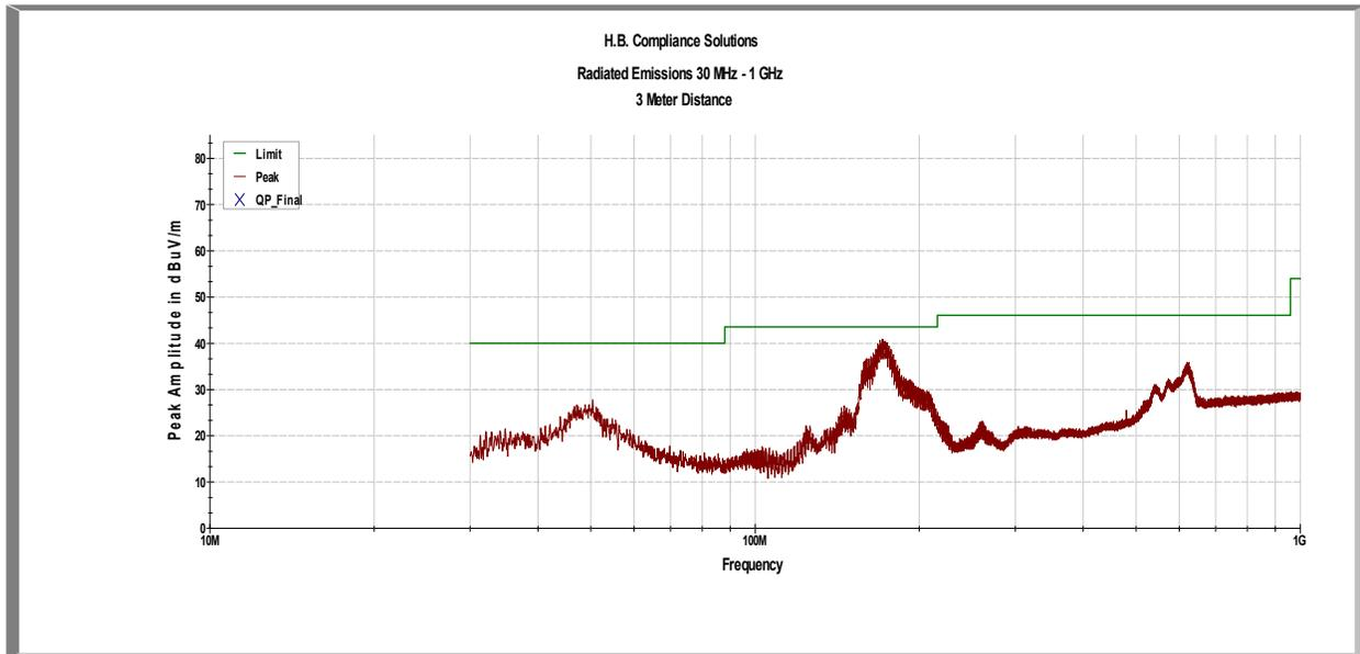
**Plot 1 – Radiated Emissions – 30MHz to 1GHz**
