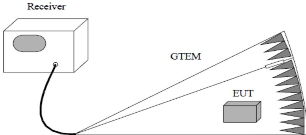
**Figure 1. Radiated Emissions Test Setup (30MHz – 1GHz)**
