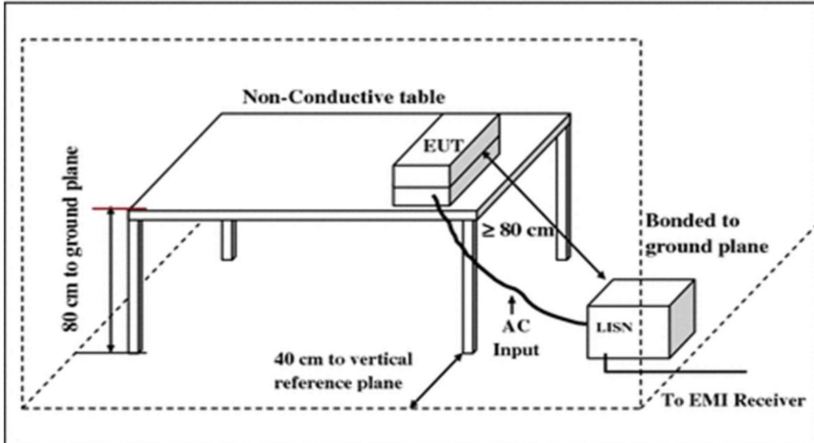
Figure 2. Conducted Emissions Test Setup
