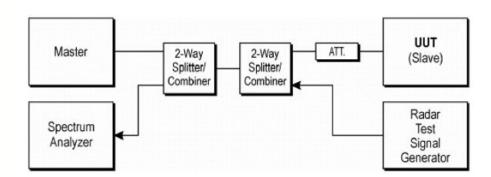
Figure 3-1. Conducted Test Setup for DFS
