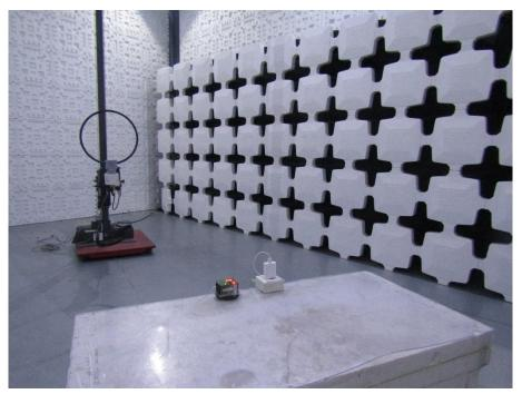
Remark: The EUT is center on the turntable, due to the edge of desk placed on the diameter of the turntable
