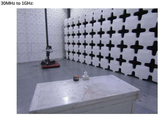
Remark: The EUT is center on the turntable, due to the edge of desk placed on the diameter of the turntable
