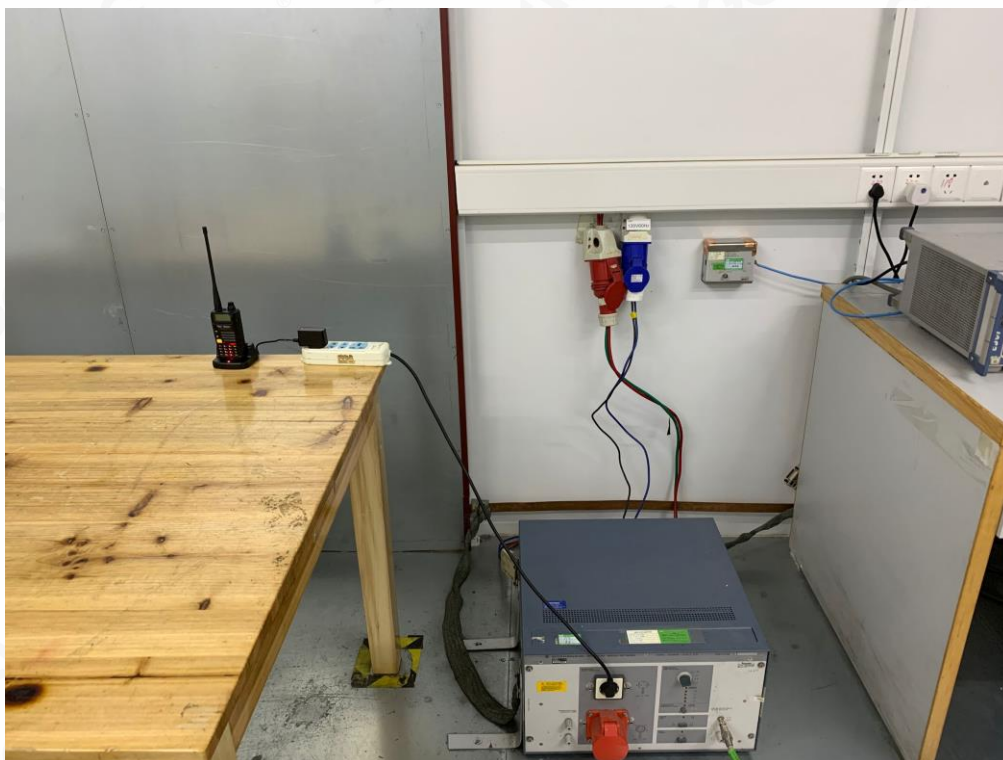
RADIATED EMISSION TEST SETUP-BELOW 1GHZ
