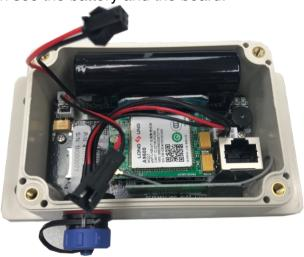
Connect the battery cable and power on the device.
