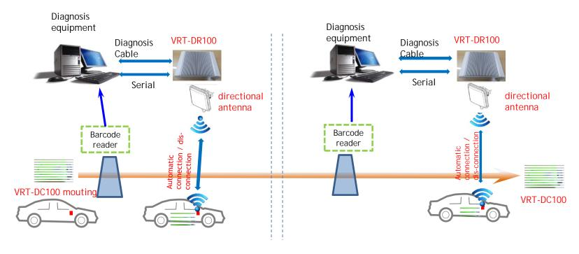
► Vehicle VIN and Barcode information matching : Barcode VIN = Vehicle VIN
