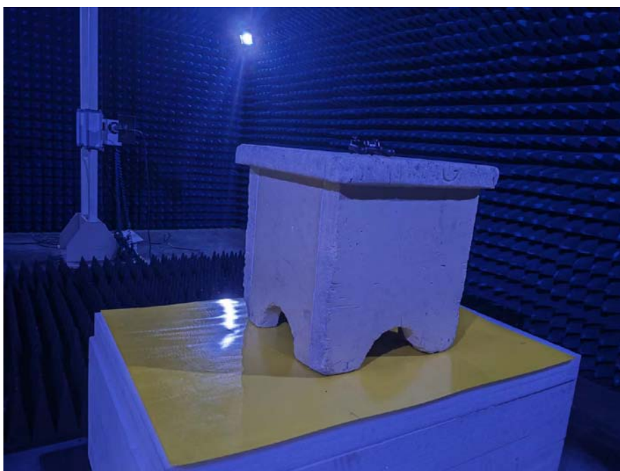
Photo of Radiated Emission Measurement (Above 1G)
