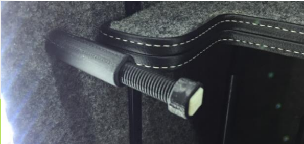
Magnet is mounted on side wall of vault to align with the Puck
