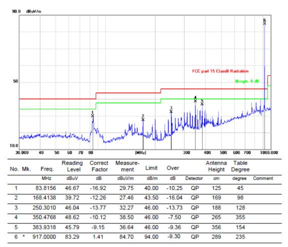
Remark: Transd = Cableloss + Antenna factor - Pre-amplifier; Margin = Limit – Level The frequency 917.0000MHz is main frequency.
