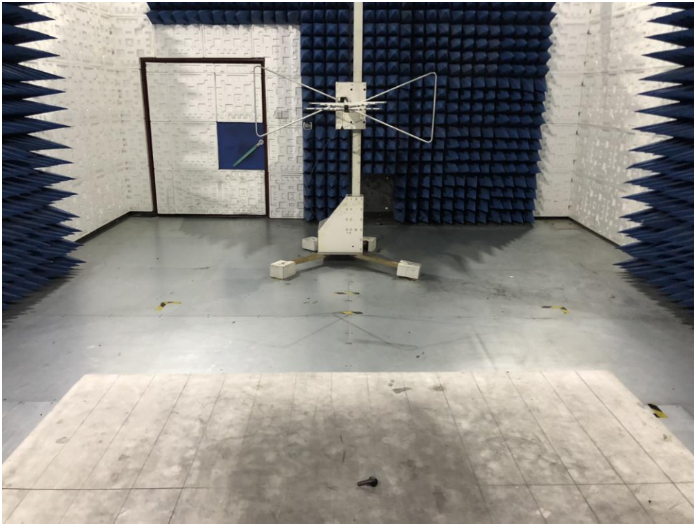
RADIATED EMISSION TEST SETUP ABOVE 1GHZ
