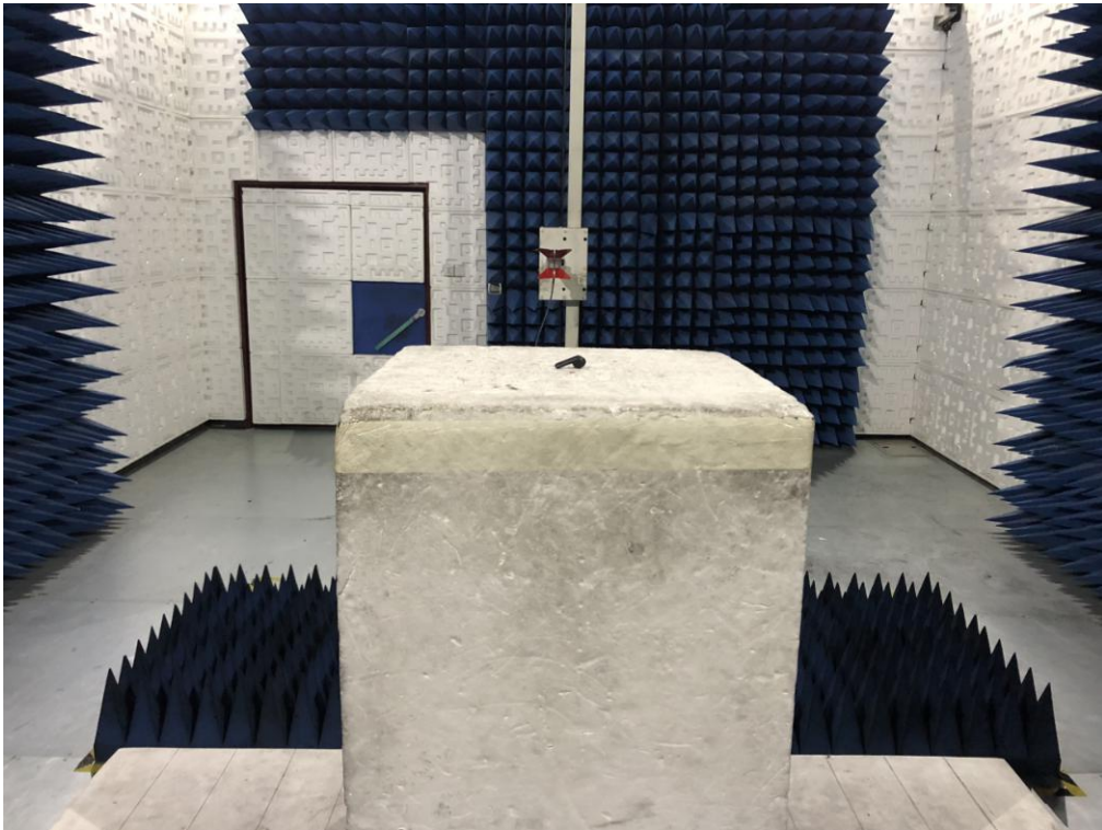
RADIATED EMISSION TEST SETUP ABOVE 1GHZ
