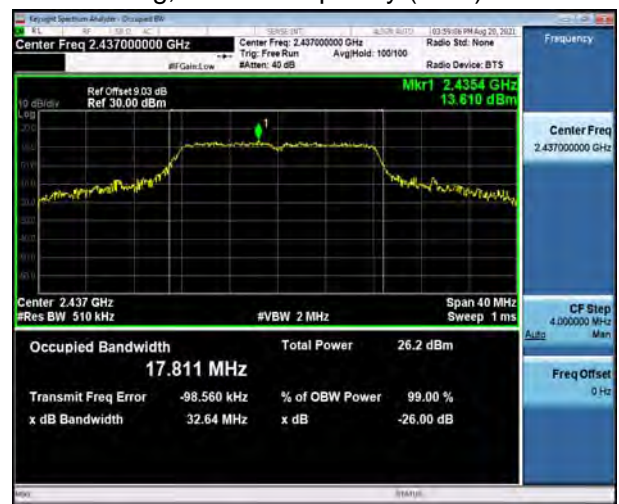
802.11g, Carrier frequency (MHz): 2437
