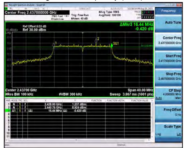
802.11g, Carrier frequency (MHz): 2437
