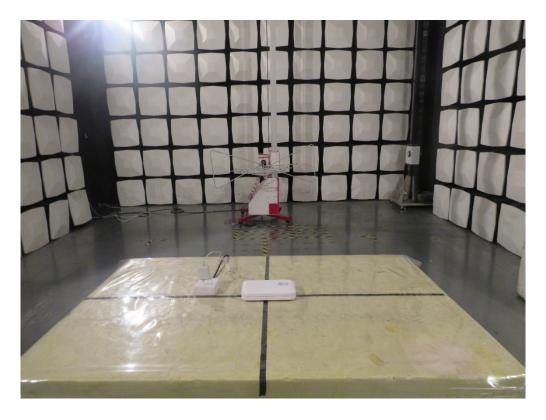
Mains Terminal Disturbance Voltage Test
