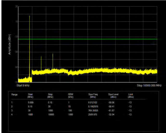
Band5 16QAM BW=1.4MHz Channel=20643 RB Size=6 Position=#0
