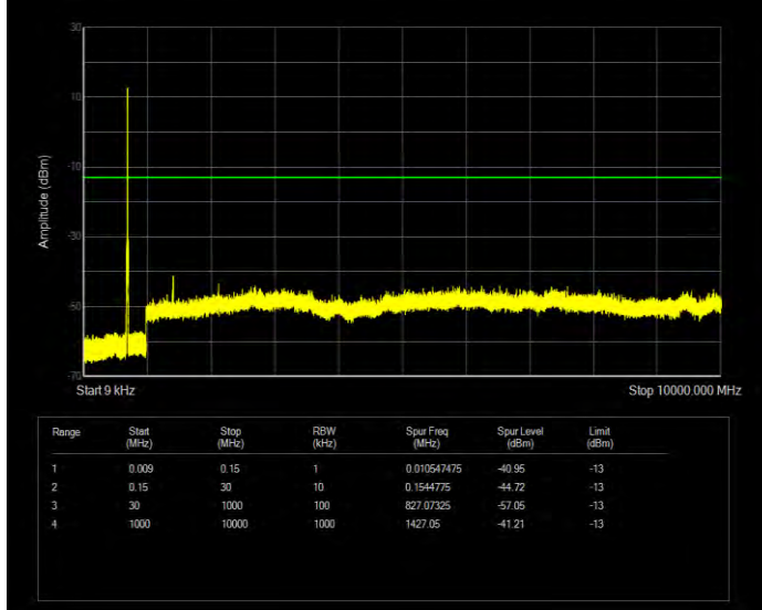
Band12 16QAM BW=10MHz Channel=23130 RB Size=50 Position=#0
