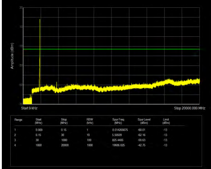
Band25 16QAM BW=15MHz Channel=26615 RB Size=75 Position=#0
