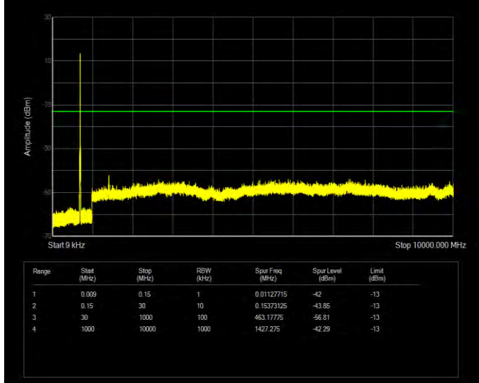
Band17 16QAM BW=10MHz Channel=23800 RB Size=50 Position=#0
