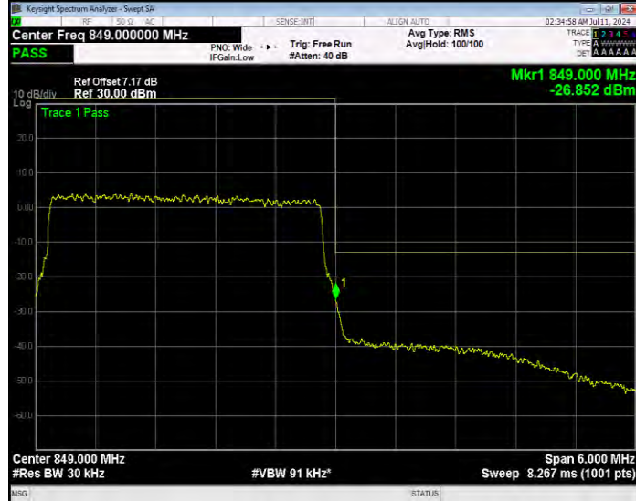
Band26(824-849) 16QAM BW=5MHz Channel=26815 RB Size=1 Position=#0 Extended
