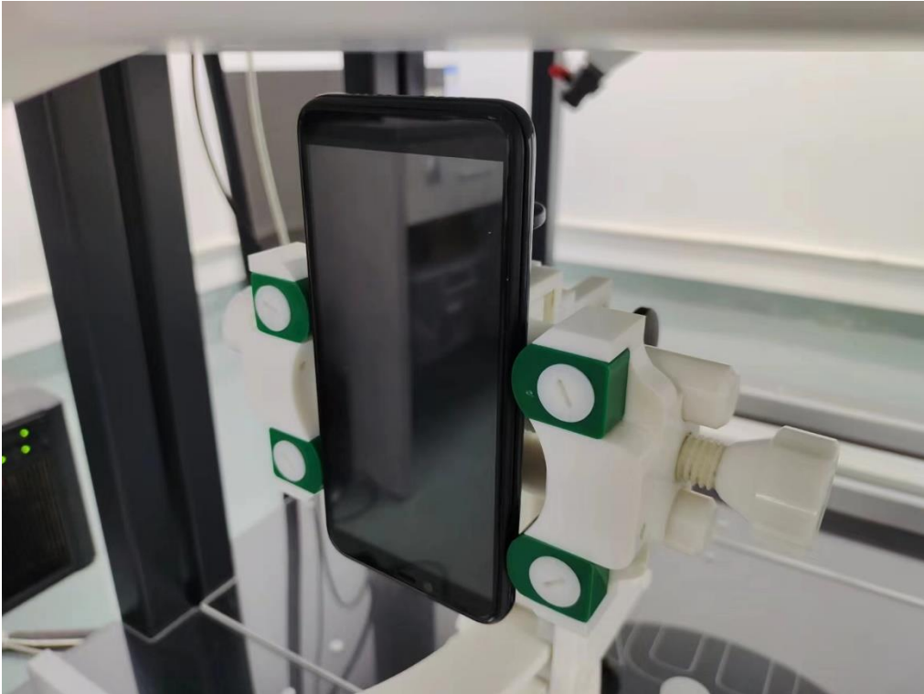
Body Bottom side (separation distance is 10mm)
