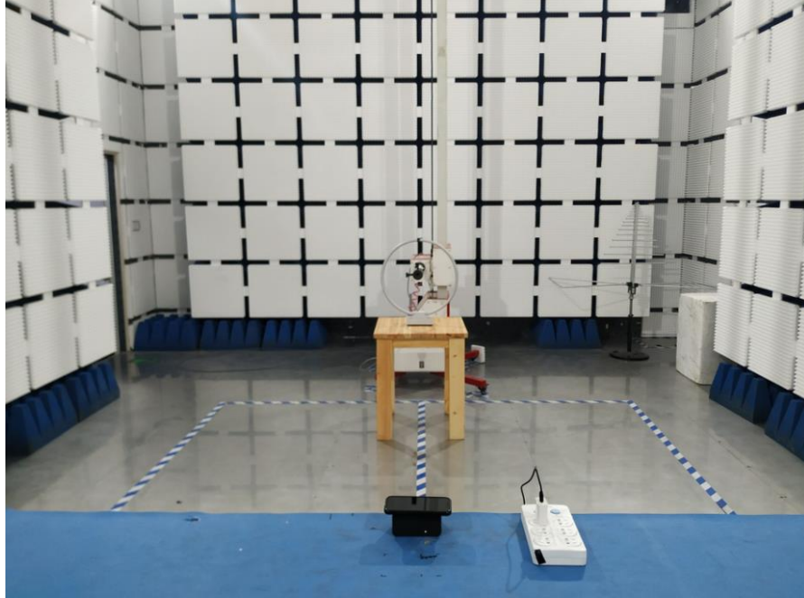
Radiated Emissions (Magnetic field Strength) (9kHz-30MHz)
