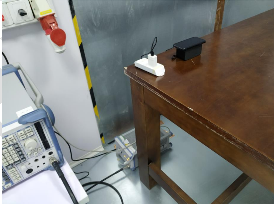
Conducted Emissions at Mains Terminals (150kHz-30MHz)
