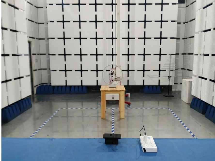
Radiated Emissions (Magnetic field Strength) (9kHz-30MHz)
