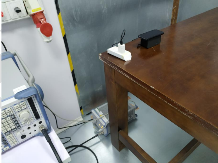
Conducted Emissions at Mains Terminals (150kHz-30MHz)
