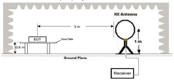
(2) Radiated Emission Test-Up Frequency 30MHz~1GHz
