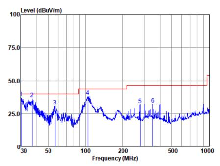
Antenna Polarity : VERTICAL EUT/Project :18695CR
