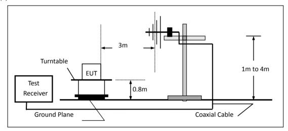
(c) For radiated emissions above 1000MHz
