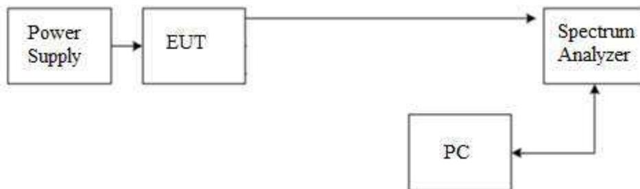
The DC supply voltage is applied using an external power supply.
