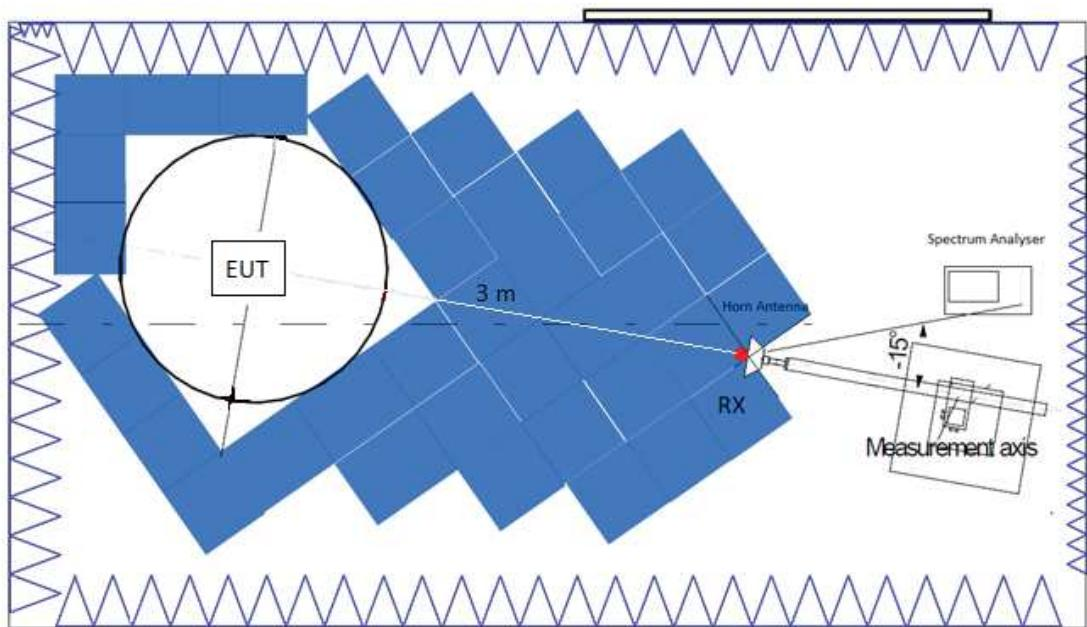
Radiated measurements setup  $f > 17 \text{ GHz}$  up to 40 GHz.
