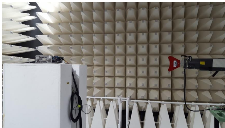
Figure B6: Radiated Emission Setup 3
